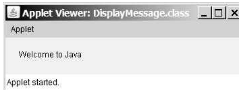
FIGURE 18.6 The applet displays the message Welcome to Java passed from the HTML page.
