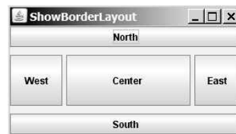
FIGURE 12.9 BorderLayout divides the container into five areas, each of which can hold a component.
